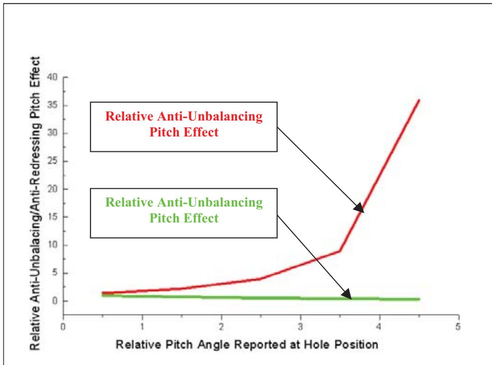
Fig. 7. The VZN shock absorber anti-pitch behaviour, relative to the standard one
