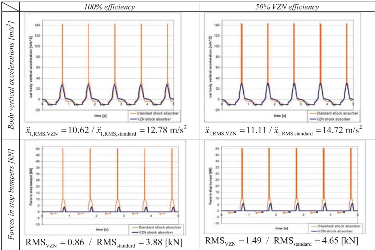
Fig. 10. Car body behaviours for road profile with amplitude 0.2m at frequency 1Hz
