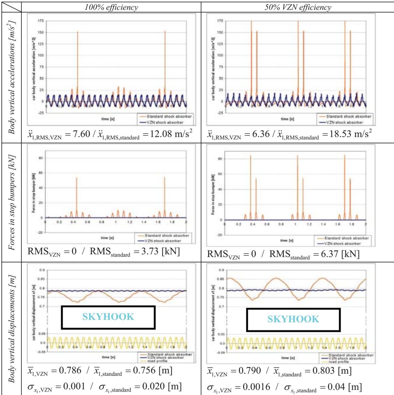
Fig. 12. Car body behaviours for road profile with amplitude 0.03m at frequency 12Hz
