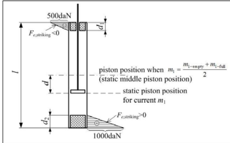
Fig. 9. The shock absorber with stopper bumpers scheme
