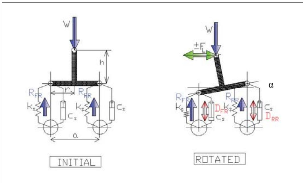
Fig. 4. The planar pitch model
