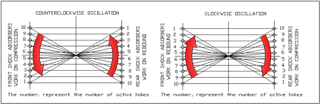
Fig. 5. The number of active holes acting on clockwise and counter clockwise
