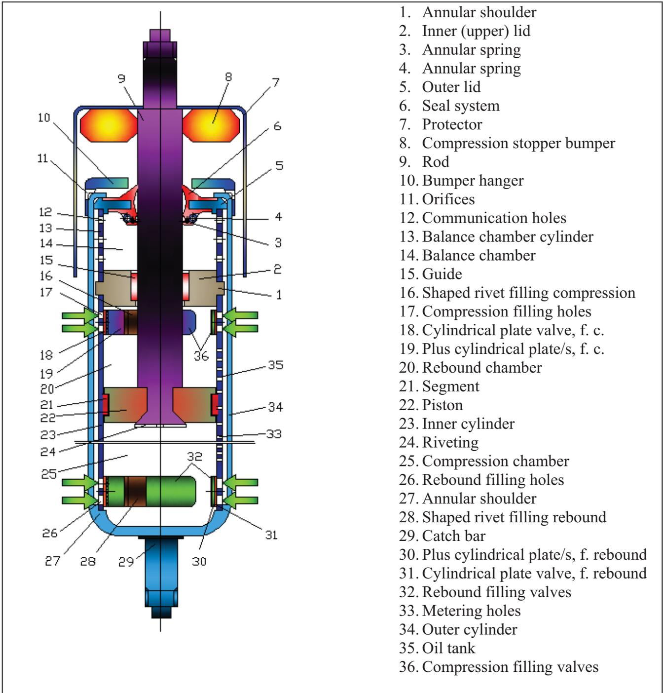
Fig. 3. The VZN –shock absorber cylindrical filling valves solution
