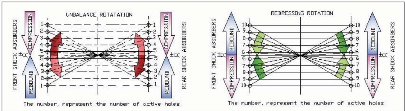
Fig. 6. The shock absorbers number of active holes acting on unbalance and redressing rotation
