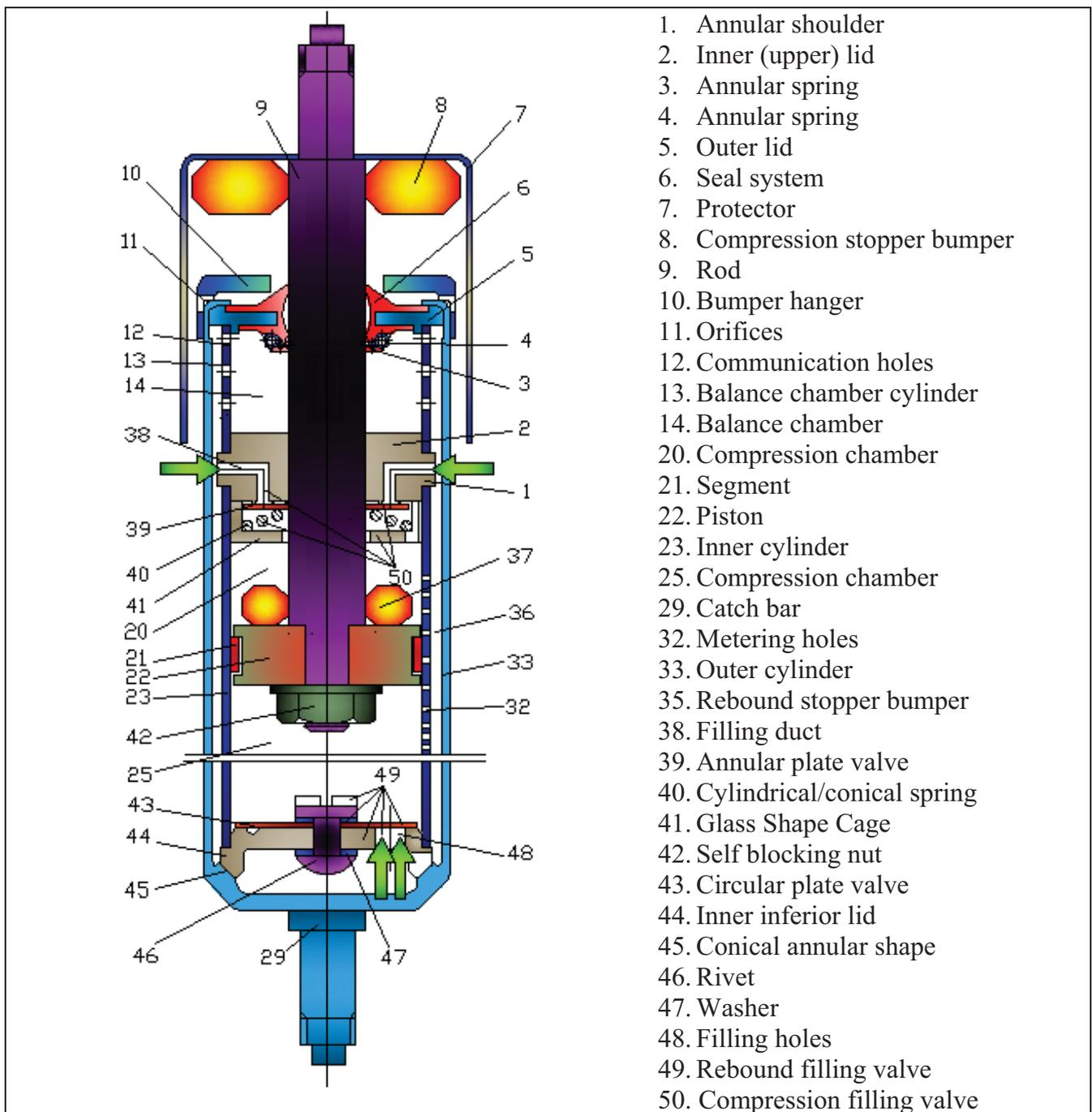
Fig. 2. The VZN shock absorber planar filling valves solution
