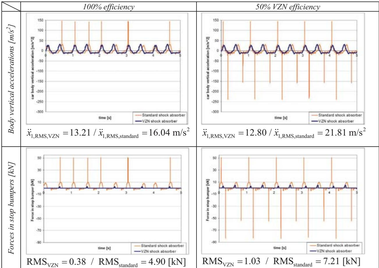
Fig. 11. Car body behaviours for road profile with amplitude 0.1m at frequency 2Hz
